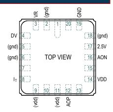
DV (input): Pin 4. Deflection Voltage. Connect to the 2.5 Volt pin for best
